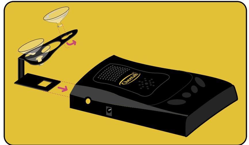
The power cord should be plugged into the cigar lighter socket for power. Any excess cable can easily be hidden underneath the glove box. Care should be taken to ensure that the power cord does not interfere with the correct operation of any airbag or other vehicle control or system. If you intend to swap your C100 between vehicles we recommend fitting an extra power cord in the second vehicle.
